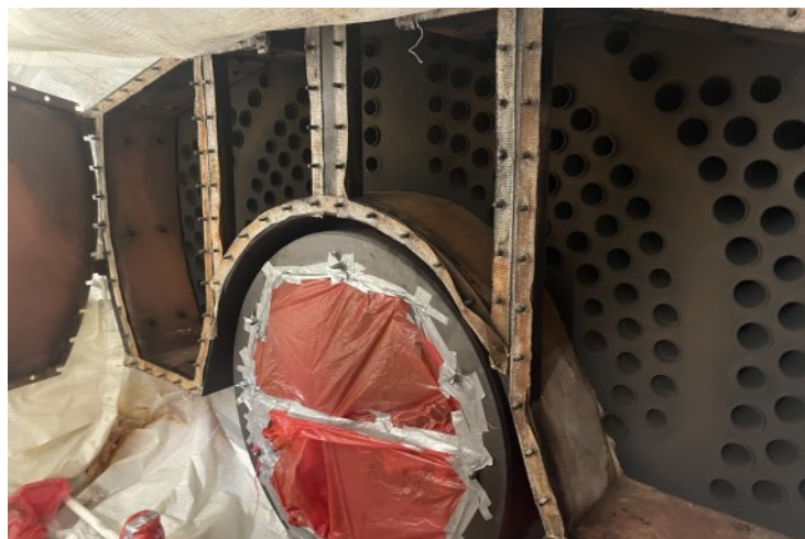
One of Waverley's boilers opened up with the tubes visible. Each tube is individually cleaned by brushing through the fine soot - a messy task!
