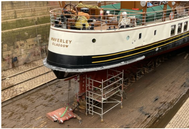
The rudder lowered down to the dock floor for full inspection of the rudder and rudder stock which was last replaced in 2018.
